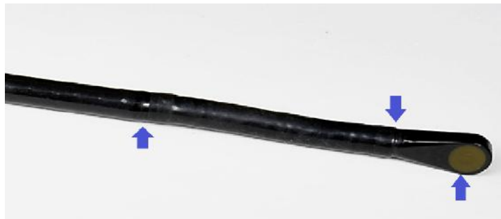
[Figure 1. TEE probe MMPT3-7 with contamination spots (arrows)]
